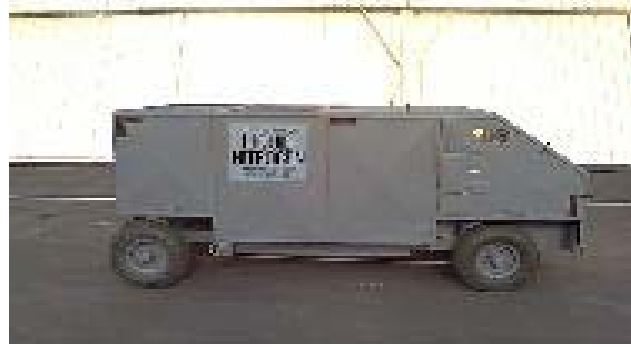
Figure 4. Nitrogen Servicing Unit
